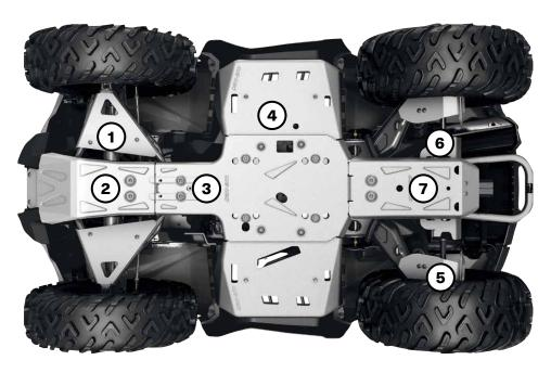
For ultimate durability and strength, all our Aluminum Skid Plates are made with  $\frac{3}{16}$ " (4.5 mm) thick High Strength 5052 H32 Aluminum.
